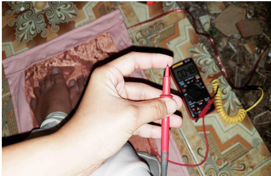
Figure 5. The measurement of skin voltage when using Earthing device resulted in 4.8 mV. Picture source by Estiningtyas
